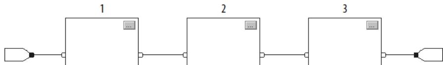
The order of execution is only relative to the blocks that are wired together. The two groups of blocks in this example are not wired together. The blocks
