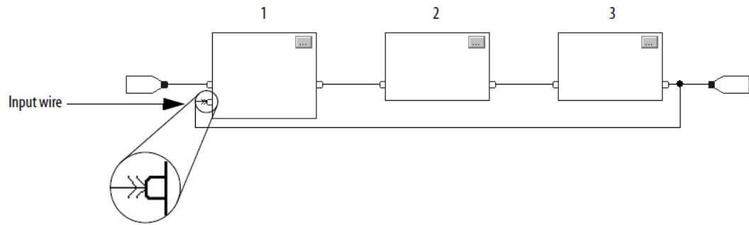
The arrow indicates that the data serves as input to the first block in the loop.
