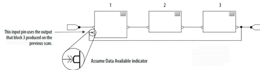
The **Assume Data Available** indicator defines the data flow within the loop. The arrow indicates that the data serves as input to the first block in the loop. Do not mark all the wires of a loop with the **Assume Data Available** indicator.
