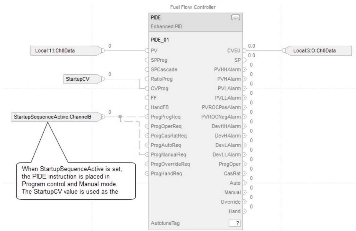
Operator request inputs to an instruction are always cleared by the instruction when it executes. This lets operator interface work with these instructions by setting the desired mode request bit. It is not necessary to program the operator interface to reset the request bits. For example, if an operator interface sets the **OperAutoReq** input to a PIDE instruction, when the PIDE instruction executes, it determines the appropriate response and clears the **OperAutoReq**.
