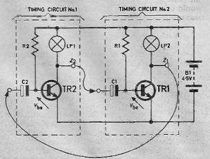
of two similar timing circuits connected so that the transistor of either circuit acts as the "switch" for the other "half". Consequently the recharging of (say) C2 via R2 determines the instant at which TR2 can switch from off to on and it is the switching on of TR2 which initiates the timing interval during which C1 can recharge via R1.
