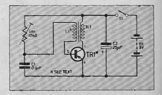
Fig. 1. Circuit diagram of the complete Simple Buzzer.
