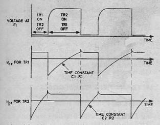
Fig. 8.2. Voltage waveforms for the astable multivibrator.
