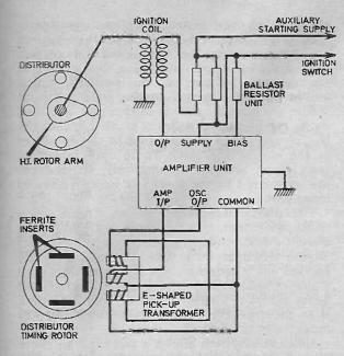
Fig. 4. A transistor assisted ignition system using a magnetic pickup.
