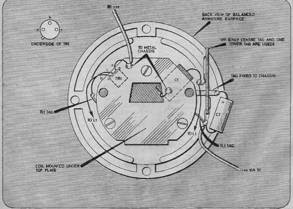
Fig. 2. Complete layout and wiring of the simple buzzer.
