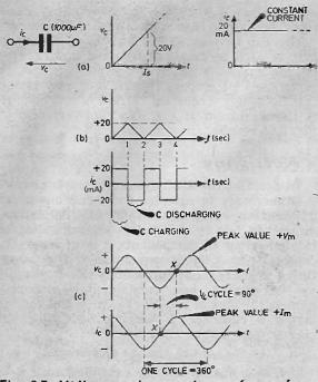
Fig. 8.7. Voltage and current waveforms for a capacitor.
