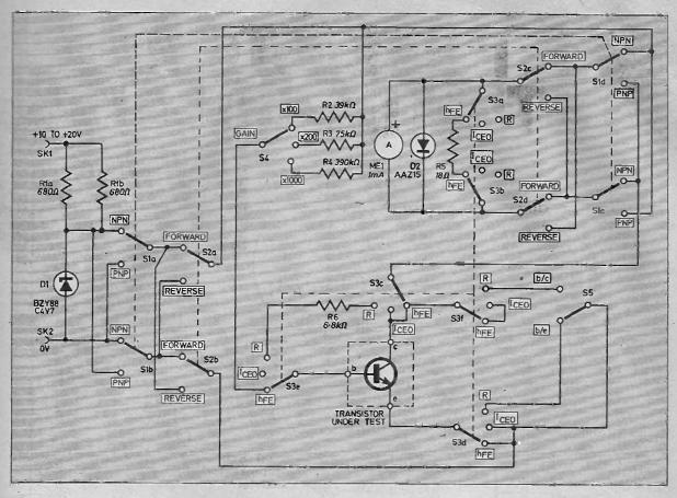
Fig. 2. The complete circuit diagram of the Transistor Tester.
