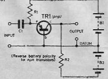
The collector current flows via R2 which is supplied with a negative voltage (relative to datum) by B2. The small base current must flow in the datum lead which is *common* to input, output, B1 and B2.
