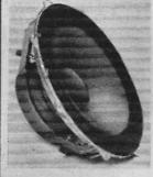
15"14A/780. Bass unit on a rigid diecast chassis. Superior cone material handles up to 50 watts RMS, and is treated to give a smooth frequency response. Resonance 30 Hz. flux density 360,000 Maxwells. Impedance at 1 kHz is 8 phms. 3" voice coil.
