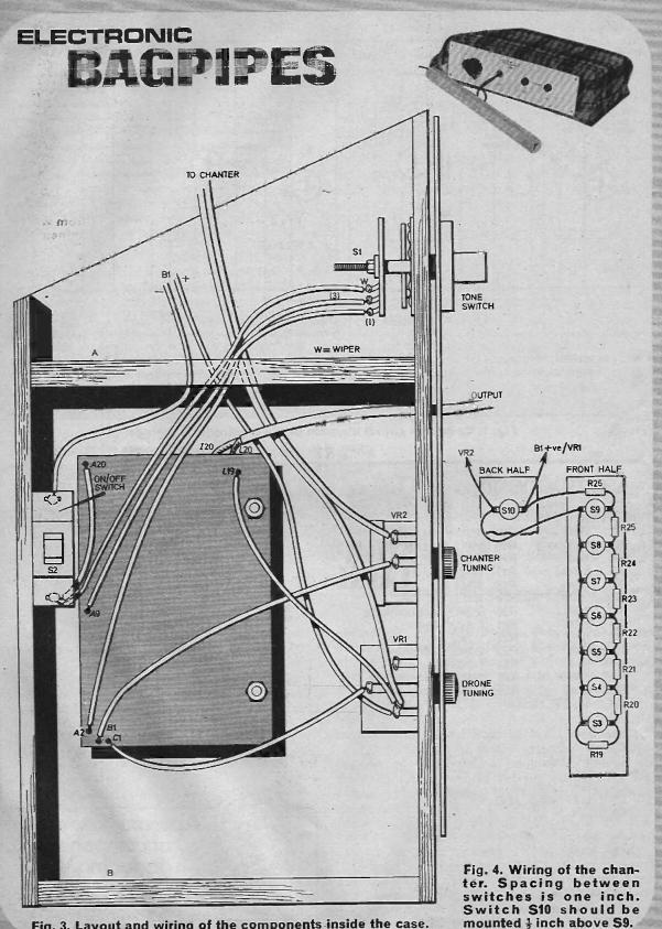
Fig. 3. Layout and wiring of the components inside the case.
