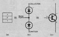
Fig. 1. (a) Schematic layer representation (b) diode representation (c) circuit symbol of an *npn* transistor.
