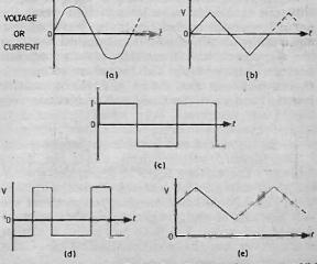
The waveform in Fig. 8.5e is not, strictly speaking, an alternating waveform, since it is always positive, but it can be considered to be made up of two parts. If we add a steady positive voltage to an alternating voltage such as that in Fig. 8.5b we can produce a waveform exactly like that in Fig. 8.5e. This idea of breaking a waveform into steady and alternating portions is also very useful.
