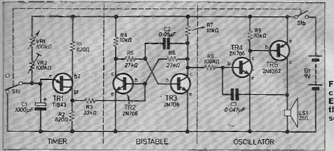
Fig. 2. The complete circuit diagram of the Egg Timer showing the three major sections.
