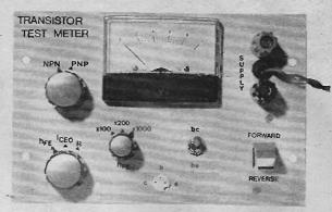
Fig. 4. Details of component positions and labelling on the front panel of the unit.
