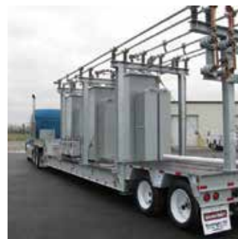
Modular Integrated Transportable Substations
