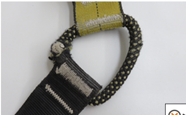
• Damaged attachment point
