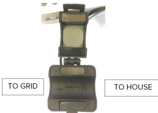
Fig. 23 Open CT showing arrow direction inside CT
