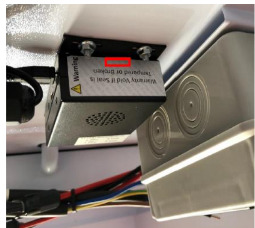
Fig 19: SD card slot location
