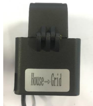
Fig. 14 Sticker on the back of CT showing correct orientation
