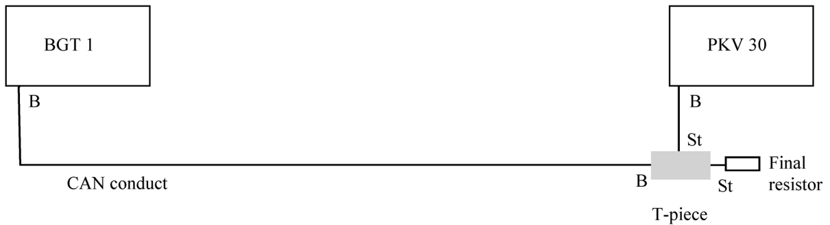
Figure 9-5: Connection Suprema Gateway CAN/MOD-BUS RTU
