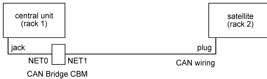
Figure 5-28: Connection CAN-Bridge CBM
