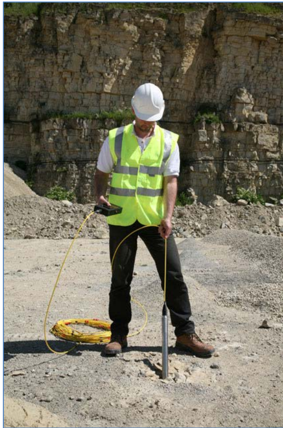
Figure 16 Rodded Boretrak system on-site
