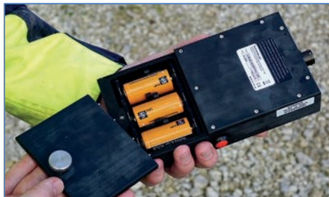
Figure 2 CDU battery compartment
