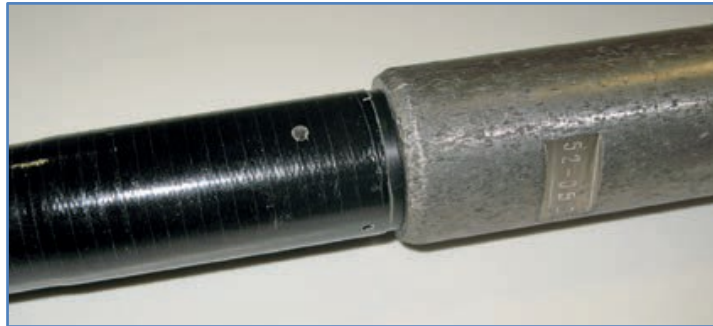
Figure 12 Ballast rod fitted to probe
