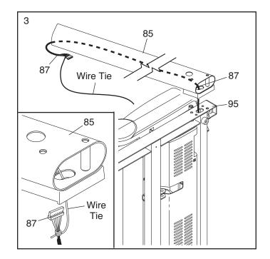
Hold the Right Upright (85) against the Base (95). Be careful not to pinch the Upright Wire (87). Insert two 3/8" x 4" Bolts (7) with two 3/8" Star Washers (11) and a 3/8" x 1 1/2" Bolt (14) with a 3/8" Star Washer (11) into the Right Upright.
