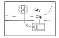
sole. After a moment, the displays will light. IMPOR-TANT: In an emergency, the key can be pulled from the console, causing the walking belt to slow to a stop. Test the clip by carefully taking a few steps backward; if the key is not pulled from the console, adjust the position of the clip.
