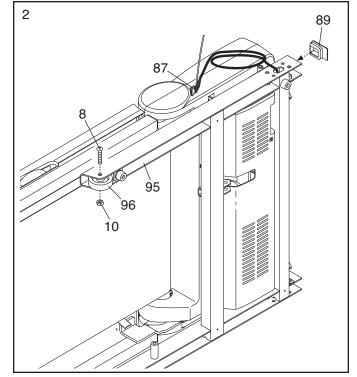
3. Identify the Right Upright (85), which is marked with a "Right" sticker. Hold the Right Upright near the Base (95) as shown.
