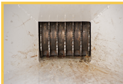
6" x 10" chipper opening to accept forked branches
