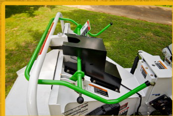
Panic Bar is a dedicated stop mechanism for the feed system independent of the feed control bar
