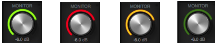
Monitor level indications (from left to right): Normal, Mute, ALT 1, and DIM/MONO
