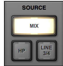
Monitor source select switches
