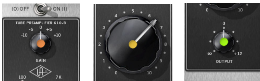
The matching color dot on the parameter in the Unison plug-in interface indicates which gain stage is being controlled by Apollo's front panel preamp knob
