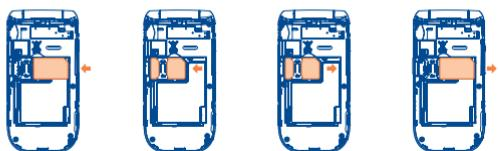
Place the SIM card with the gold contacts facing downwards and slide it into SIM card slot. Make sure that it is correctly inserted. To remove the card, press and slide it out.
