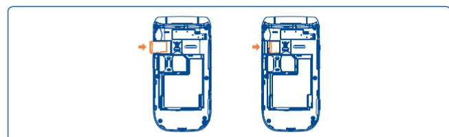
Insert the microSD card with golden contact facing downwards into the slot until it is locked. Gently push the memory card until it is unlocked.
