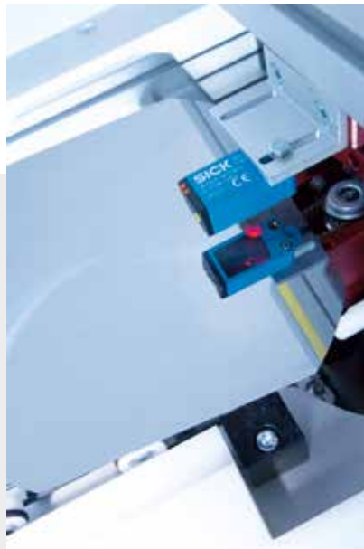
Special sensor variants reliably detect both the strongly reflective wafers as well as the cells that absorb the light in the production of solar cells.
