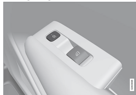
Button with indicator light for locking/unlocking in rear door.
