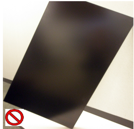
Never rest the LCD on a corner!
