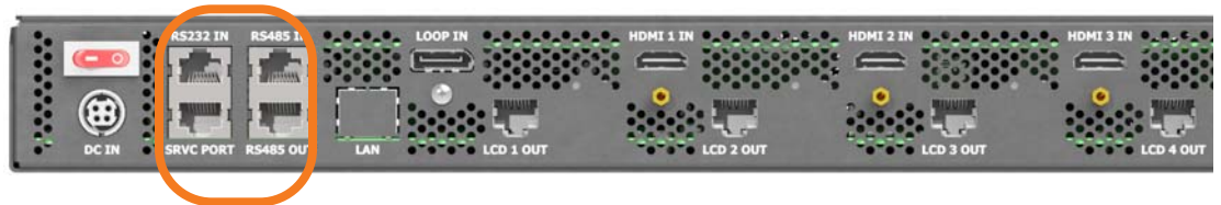
RS232 port connection is on the Quad Controller module. Only connect to Quad module A or the connection won't work.
