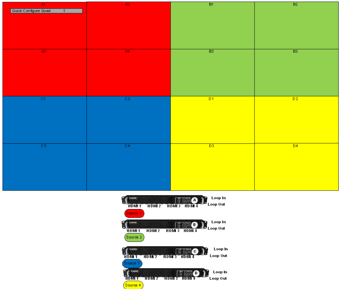
4 x 4 Matrix with one source per Quad controller module.
