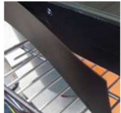
Million peeling away from bezel (ERO units only)
