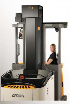
The sloped power unit design and flexible seat positions give the operator a clear view of the aisle improving maneuverability and operation in and out of the aisle.
