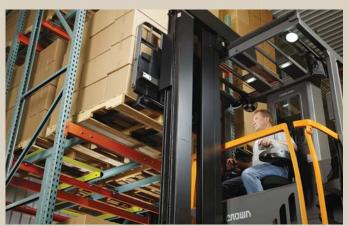
PUSH BACK RACK: Powerful traverse motor allows multiple pallets to be "pushed back" on rolling carts for increased pallet density.
