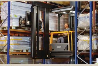
**LONG LOADS: Extended load handlers** on the TSP Series can handle loads in excess of 100" such as furniture, construction materials or mattresses (as shown above). The optional **fork positioner** helps in applications with varying pallet sizes.
