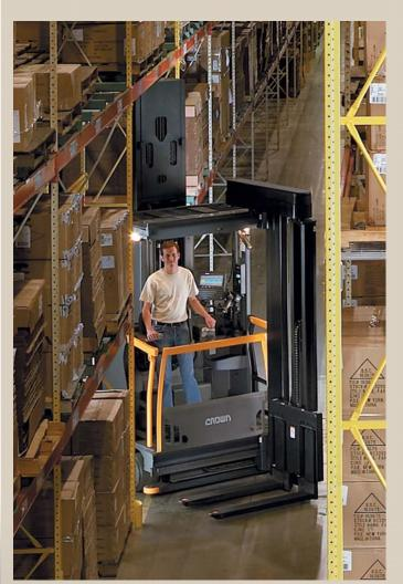
NAVIGATING LOW AREAS: Crown's TT Mast Option provides extreme lift heights and low collapsed heights all in one. This allows very tall trucks to easily navigate tunnels (as shown above) and other obstructions such as conveyors and mezzanines.
