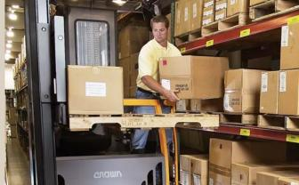
PICKING: Sturdy steel side gates and clear front rail reduce the need for operators to bend or lean when retrieving product from the rack or placing it on a pallet (as shown). In addition, the rails can be used to support the weight of the product as it is transferred from rack to pallet.
