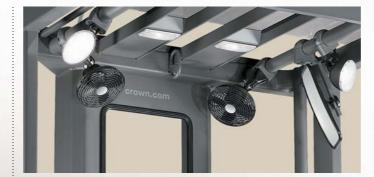
Work Assist® Accessories add even more productivity to each shift. Standard accessories include LED work-lights, dome lights, mirrors, fans and more. Additional accessories are available as options based on your application and operator requirements.
