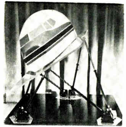
Tilt. New generation of simulators like this one from Link have double the number of axes of motion freedom.
