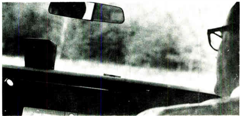
Follow me. Experimental Route Guidance System provides head-up display mounted on dashboard to give directions.
