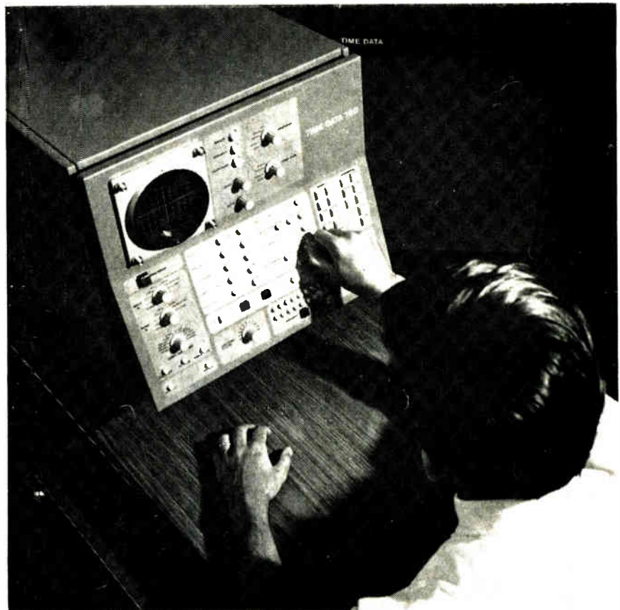
Excavator. Time/Data Corp.'s special-purpose Fourier analyzer extracts signals buried in noise.
