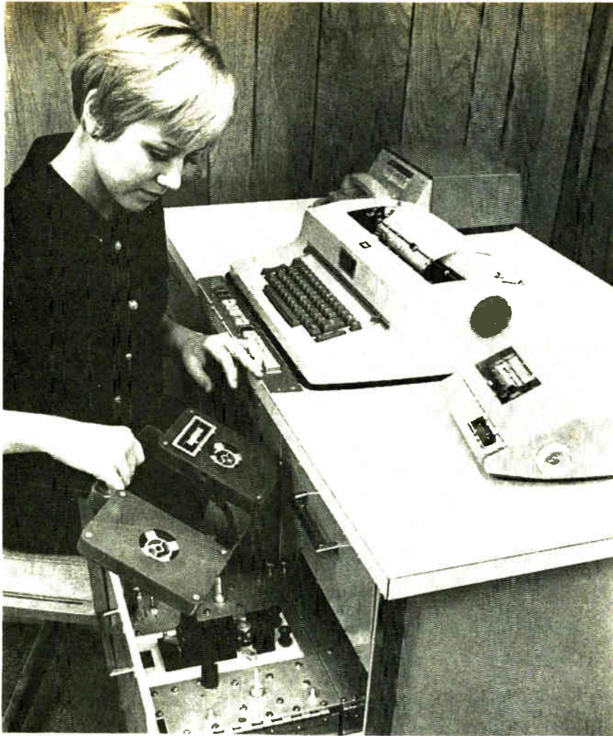
In and out. The removable magnetic tape cartridge in Communitype's data communication system has capacity of 180,000 characters or 30,000 words.
