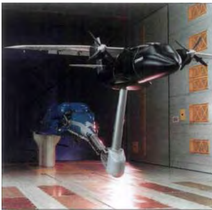
Wind tunnel testing of a model of the DORNIER 328.
