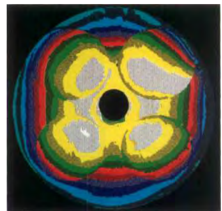
Holographically measured deformations, due to the internal pressure in the combustion chamber of a 4-valve cylinder head.
