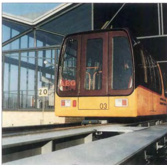
The M-Train developed by AEG is a fully automatic local public transport system.
