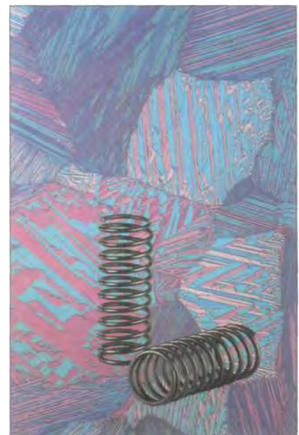
The crystalline structure of a shape memory alloy (magnified by 270:1). The possibilities of using alloys which can "remember" their original form are being researched. For example: spiral springs.
