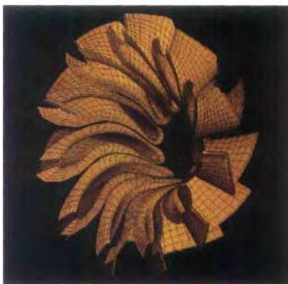
Milling pathways for NC manufacture of a turbocharger-turbine wheel: the turbine wheels are developed via a closed data transfer, which extends from the aerodynamic design right up to manufacture.
