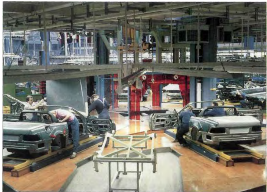
Star-shaped assembly stations for the new roadster allow economically favorable fitting of the hydraulic lines, cable harnesses and folding soft-top.
