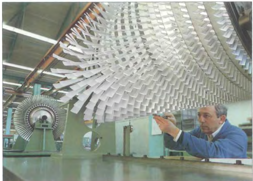
On this 17-stage axial compressor rotor of an aero-engine, the tip clearance of every blade is measured and documented.
