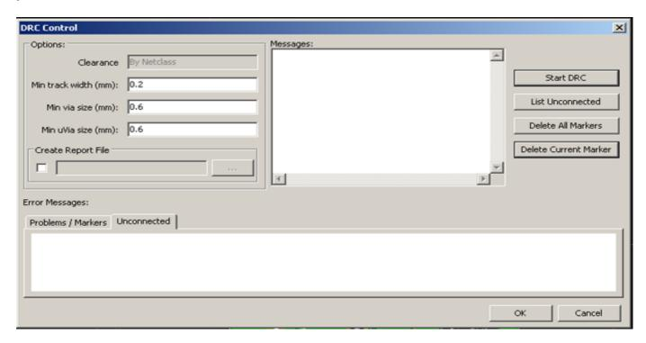
set the minimum track to 0.2 mm, minimum via to 0.6 mm and minimum uVia to 0.6 mm, then StartDRC, if errors show please fix them, until no error is displayed.
