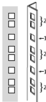
Figure 8: Hole distribution on 19" rack
