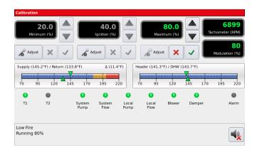
The MAXIMUM % value is used to set the maximum fire rate of the boiler. To adjust the Maximum fire rate of the boiler, press the Adjust button under the Maximum (%) value shown in the display. The percentage value will turn green. Then use the arrow keys to adjust the value up or down. Adjust it using the arrow keys and then press the green check key to save the value. Press the 'X' key to discard the setting.
