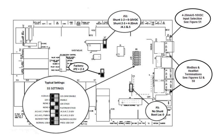
S5 Dip switches 1,5,7,8 set the Outputs of the J4 Connector.
