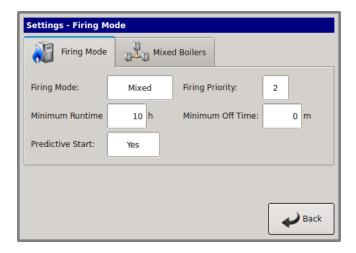
As long as the start condition for Priority 1 is met, all boilers in the PRIORITY 1 set will fire based on runtime. Once all boilers in the PRIORITY 1 set have fired, the PRIORITY 2 set of boilers will fire based on runtime.
