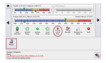
The touchscreen displays a visual flow fault and the control will annunciate an audible fault. After ten minutes, if the demand is still present, the boiler will retry to start the pumps to achieve flow and start the boiler. If there are other boilers on the network the Master will attempt to start one of them.
