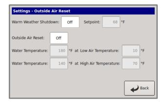
The chart depicts what the water temperature setpoint will equal with a corresponding outside air temperature. At an outside temperature of 10F and below, the water temperature setpoint will be limited to 180F. With an outdoor temperature of 70F and above, the water temperature will be limited to 140F. The water temperature setpoint will track along the charts plotted line with corresponding outside temperatures.
