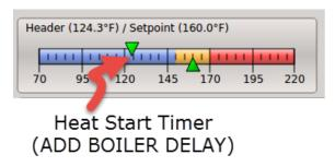
When the Header temperature is above the band (Yellow), the HEAT STOP TIMER (Shed Boiler Delay) is used to stop/shed boilers.
