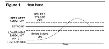
The control algorithm is based upon a Heat Band, at the center of which is the setpoint. While below the Heat Band, boilers are staged on and modulated up until the Heat Band is entered. Once in the Heat Band, modulation is used to maintain setpoint. Boilers are shut down only when the top
