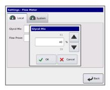
To maintain a minimum flow through the boiler, the "Flow Prove: GPM" is adjustable. Enter the minimum flow that the boiler is to prove and operate above, then select "OK".
