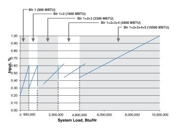
So, for the first 1800 MBTU of load, the combustion efficiency is maximized by running the (2) CK Series boilers from low to middle input rates. Running the (2) CK 1500 boilers first, also has the added effect of minimizing the return water temperatures of <140F from reaching the non-condensing boilers.
