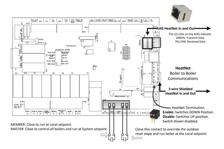
Figure 49 Heating Methods 2 and 4: AA-High Fire and High/Low, Master or member boiler
