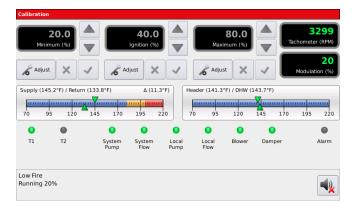
Be sure to set this switch back to NORM when the calibration is complete, otherwise no external control inputs will work (except T1-T2), the display will always indicate CALIBRATE and some of the runtime temperatures will not be displayed.
