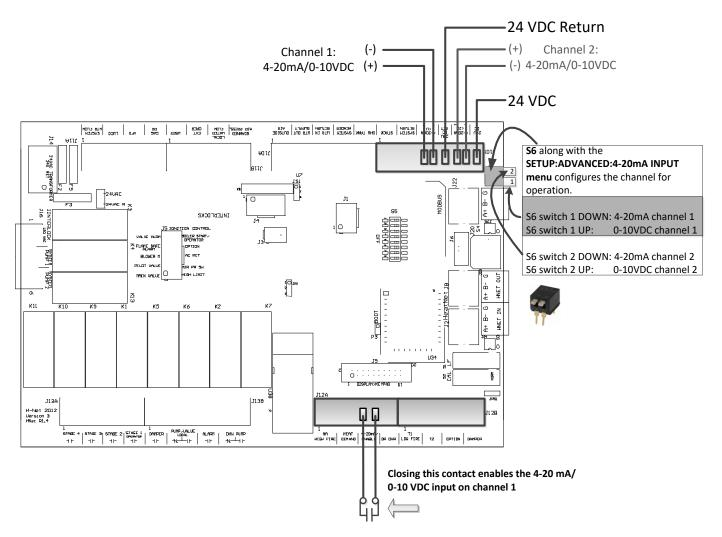
This Method allows direct modulation of the boiler based on a 4-20 mA control signal. A control capable of transmitting a 4-20mA/0-10 VDC control signal for the purpose of modulating a boiler and to control a common system temperature must be used with this method.
