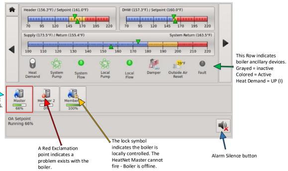
**Boxed Boilers indicate** Boilers that are recognized by HeatNet
