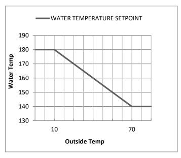
The above chart shows how the water temperature setpoint changes with the Outside air temperature. The four values of 180, 10 and 140, 70 are the default values:
