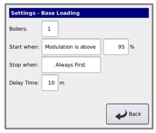
If a MINIMUM OFF time of the Base Load boiler is needed, the Base Load boiler will share the MIN OFF TIME of the boiler controlling it. If the base load boiler was running and shuts off, the MIN OFF TIME will need to expire before the boiler can start again. Once this time expires, the DELAY TIME also needs to expire to start the boiler. This will help in
