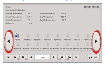
The Center middle annunciator shows icons of the boilers in the system/standalone with graphics indicating if they are firing. The large arrow buttons on the left and right of the boiler icons allow the viewing of the control state.
