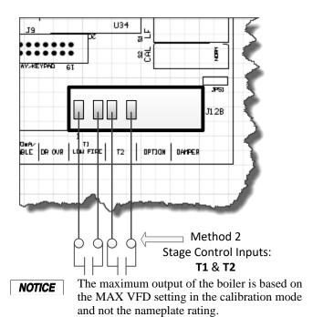
The AA, HEAT DEMAND (LOCAL) input, the H-Net, the 4-20 mA input will all override the stage control inputs.
