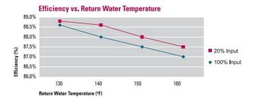
Figure 8 Typical efficiency of Torus boilers
