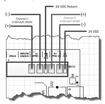
Figure 43 4-20 mA enable connection
