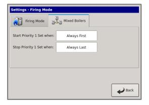
Once the Mixed Boilers menu has been entered, the firing order and stop order of the Priority 1 boiler set can be selected based on up to (3) conditions in the conditional settings menu. All conditional settings apply to the Priority 1 boiler set. When the conditional settings do not apply to the Priority 1 set, the conditional settings will apply to the Priority 2 boiler set.
