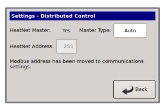
A **MASTER TYPE** is required when using DHW. Its setting is located under the **DISTRIBUTED CONTROL** menu. Any time its setting is changed, a power cycle is required. The menu choices are:
