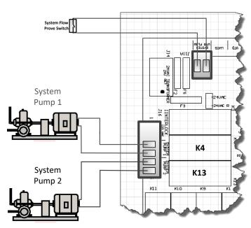
The summer pump jog is a special feature that can be selected when the system is in summer shutdown (OUTDOOR RESET). The jog allows the system circulator pump(s) and the local pump to run for the system pump purge time once a week. It can be set to any day of the week and will occur at 12:01 AM. If (2) system pumps are present, and after the first pump finishes its post purge, the second one will start and the first one will stop.
