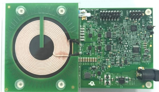
Figure 1. WCT-15W1COILTX reference board
