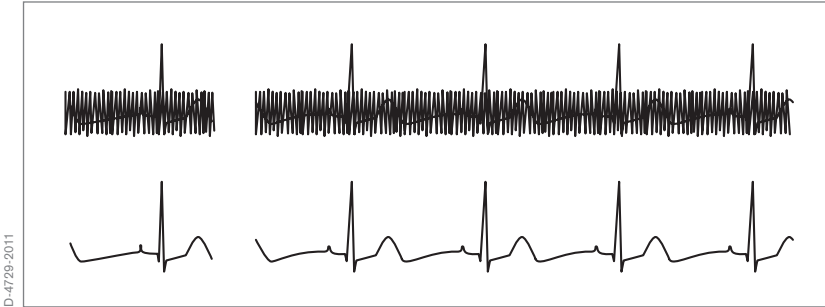
Figure 41 - Typical power supply interference
