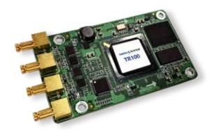
TR100, a new generation of receiving card with coaxial connectors as the transmission media, features higher pixels drive capacity up to 384×384, and supports 1.0/2.3 connector which ensures more reliable system connection and data transmission. Benefiting from the SerDes technology, TR100 has the lower latency feature (1 frame).
