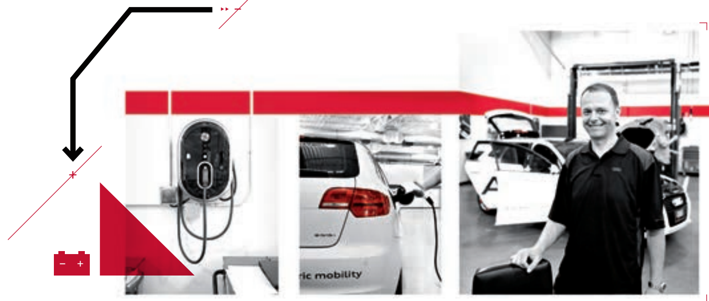
A 230-V standard charger will need six hours to recharge the car fully.
