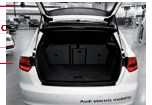
With clever battery-pack placement in the trunk, it still has an ample 26.5 cu ft of cargo space (with rear seat folded).
