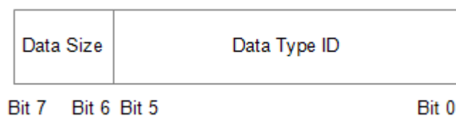
Figure 19 – Sensor Data Descriptor field structure
