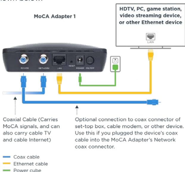
Figure 3. MoCA Connection for a Device
