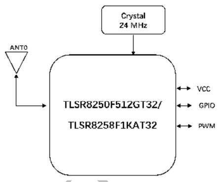
Fig 1 System Block Diagram
