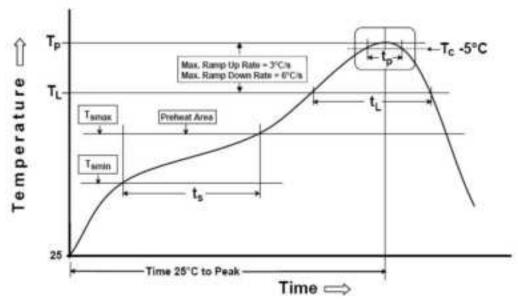
Fig 13 Furnace temperature curve
