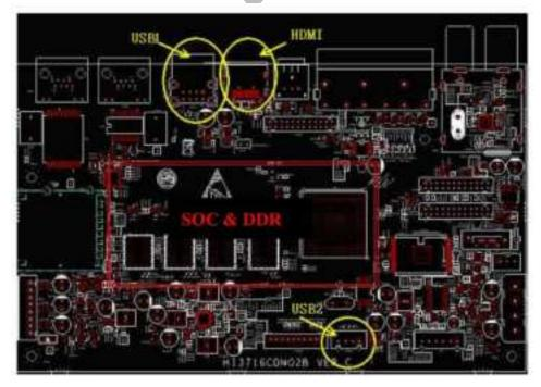
Fig 12 Main chip and DDR interference
