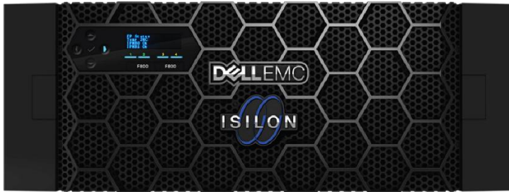
Figure 2 Isilon H500 / F800 chassis, containing four storage nodes
