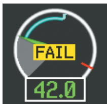
Engine Failure Indication
