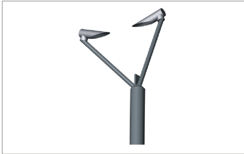
Figure 8-2. Look-down forward-scatter meter
