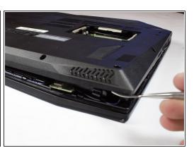
Carefully remove the back shell from the device working your way around all the edges.
