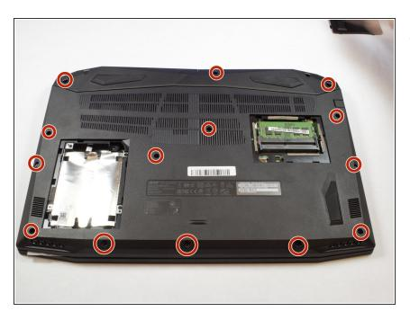
Use the Phillips #0 screwdriver to remove the 9mm screws holding the back cover in place.
