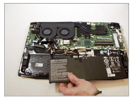
Remove battery from device.
