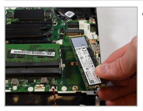
Slide the SSD out of its slot.
