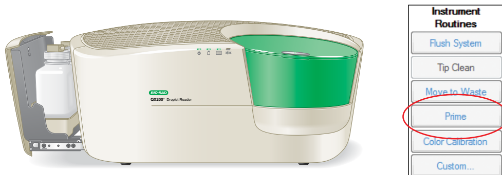
Fig. 26. Replacing droplet reader oil and removing waste. Slide out the carriage containing the droplet reader oil and waste receptacles to remove and replace the bottles (left). After replacing oil, click Prime to fill the lines; other instrument maintenance routines are for use by field specialists only.
