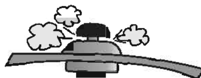
Figure 6. Overpressure Valve Releasing Steam
