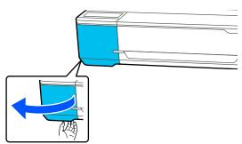
Loosen the screw holding the cutter in place using a cross-head screwdriver and pull the cutter straight out.
