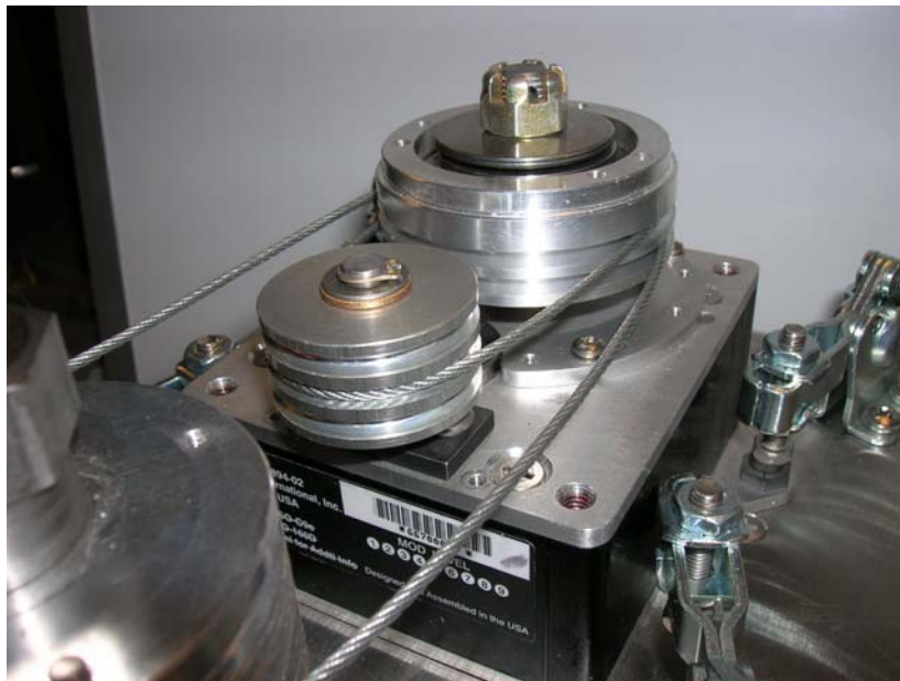
Figure 3-19. Cable wrapped around unit upper slot
