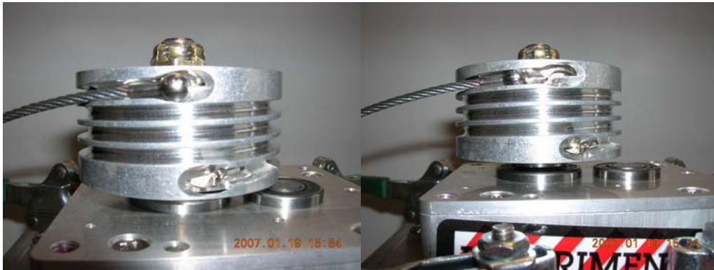
Figure 3-10. Inserting 3/32 cable in the unit capstan.
