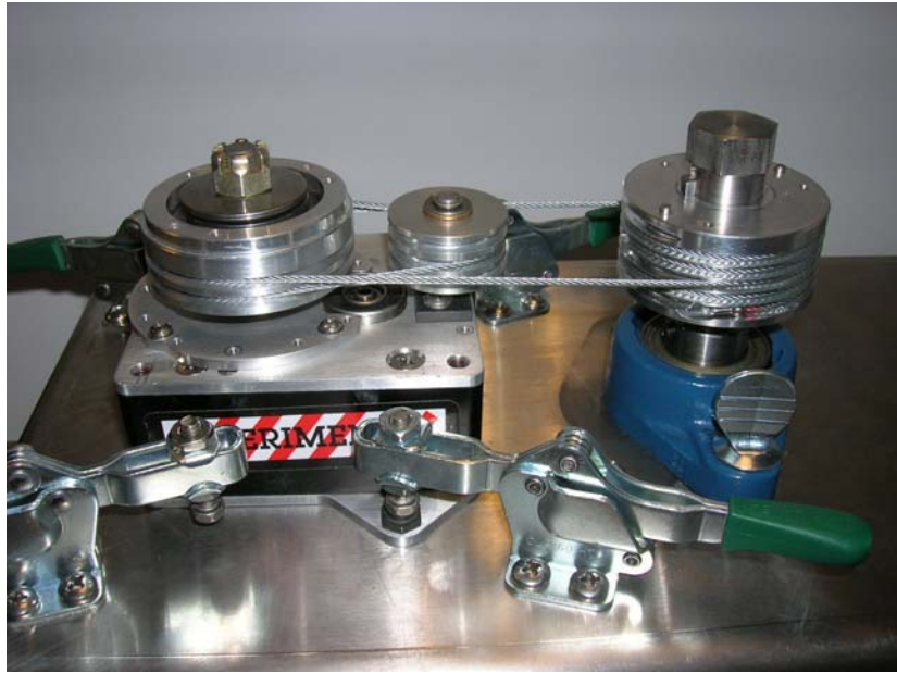
Figure 3-22. Slack taken up, capstan centered
