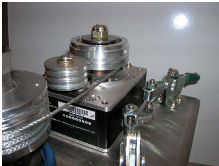
Figure 3-17. Cable wrapped 2.5 times, going across to unit capstan lower slot
