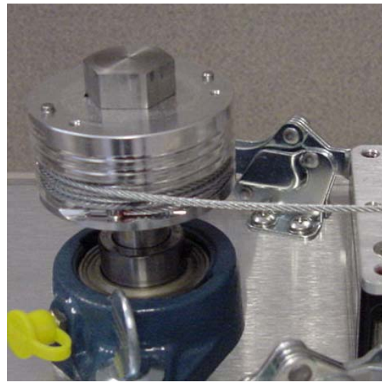
Figure 3-7. Cable Placement (fixture capstan)
