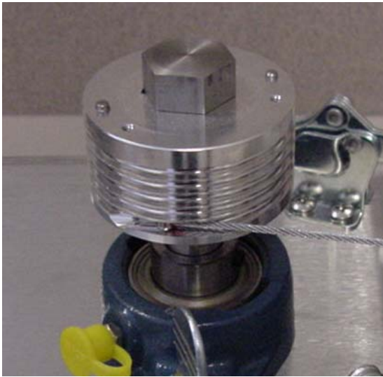
Figure 3-6. Cable Placement (fixture capstan)
