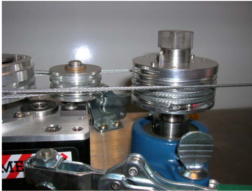
Figure 3-20. Cable routed to fixture capstan
