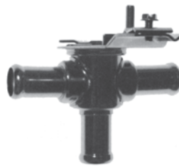
26-0043 Heater control valve 5/8" 3-way. Inlet from bottom when bracket on top*. Pull for water flow to left side.
