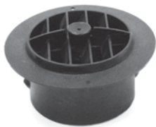
23-0100 Rotates and closes comes with 4" hose adapter (ABS) . Four screw holes at Ø 4.93" (125.2mm) Used in the RV and motor home industry.
