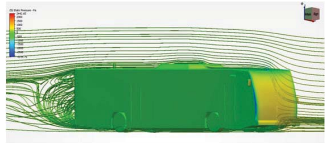
Aerodynamics analysis of a transit bus
