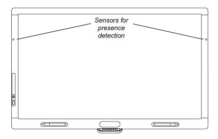
The interactive flat panel has two presence detection sensors on its frame that can detect people up to 16' (5 m) away when the interactive flat panel is in Standby mode.
