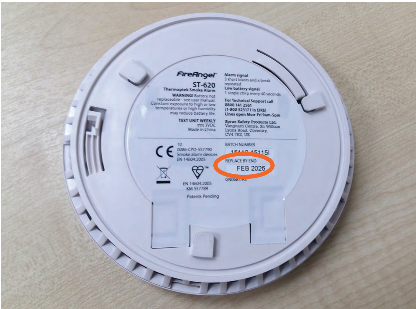
FIGURE 3: Example of the rear of a smoke alarm, identifying an expiry date.
