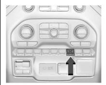
If equipped, there is an available PTO switch in the auxiliary switchbank in one of the right side positions.
