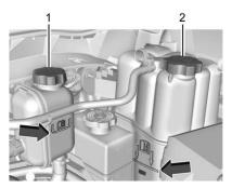
Slowly fill the coolant surge tank (2). Do not let the coolant level go above the indicated mark in the tank until after the engine comes to operating temperature in Step 4.
