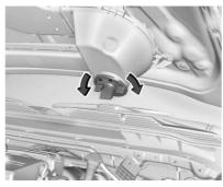
Turn the dust valve counterclockwise to remove from the front intake air duct. Check it for debris and clean out if necessary.
