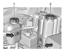
The low temperature cooling circuit coolant surge tank (1) is in the engine compartment on the driver side of the vehicle. See *Engine Compartment Overview*
