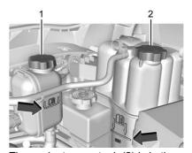
The vehicle must be on a level surface. When the engine is cold, the coolant level should be at the indicated mark.
