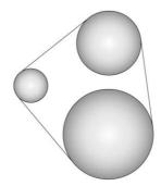
Fan Drive Belt Routing (Secondary/Auxiliary Drive)
