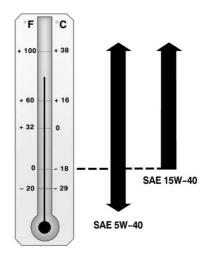
When it is very cold, below -18 °C (0 °F), use SAE 5W-40 to improve cold starting. These numbers on the oil container show its viscosity, or thickness.
