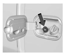
The blue DEF cap is behind the fuel/DEF door. Do not remove the fuel and DEF caps at the same time. Fill diesel fuel and DEF independently. Turn the DEF cap counterclockwise to remove.
