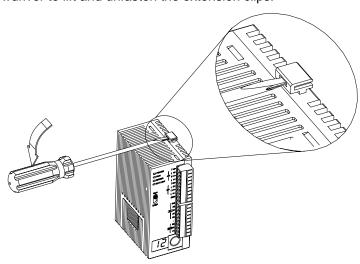
Connect the ELC-COPBDP to the extension port of the ELC controller and fasten the extension clips.
