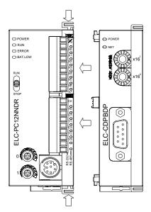
Plug the PROFIBUS connector into the socket of the ELC-COPBDP, and tighten the screw to secure the connector.
