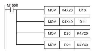
This program example copies the 4 bytes data from X20-X57 that are transmitted by the Profibus-DP master to D10 and D11 registers in the ELC controller. It also copies ELC register D20 and D21 to Y20-Y57. These 4 bytes data are sent to the Profibus-DP master.
