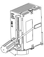
Use a screwdriver to lift and unfasten the extension clips.
