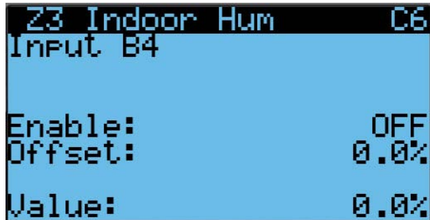
FIGURE 38 Enable/Disable Zone 3 Indoor Humidity Sensor
