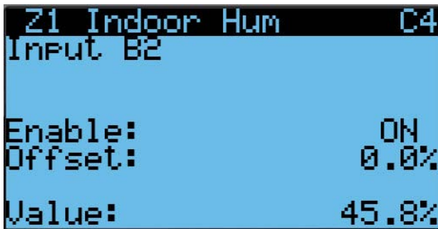
FIGURE 36 Enable/Disable Zone 1 Indoor Humidity Sensor
