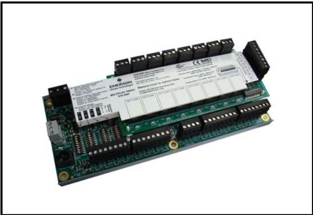
Figure 5-4 - RoHS MultiFlex Combination Input/Output Board (Side View)
