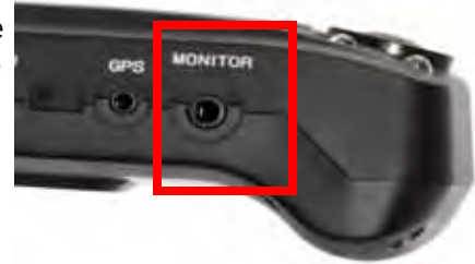
Figure 2.2 Monitor out port on the side of the Road Warrior.
