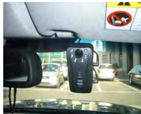
Figure 1.7 Secure Road Warrior to the right side of your rear-view mirror to prevent viewing obstruction.
