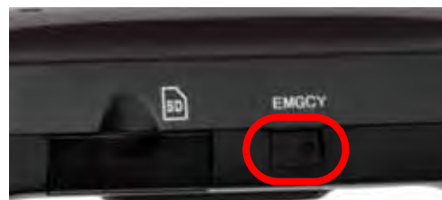
Figure 1.9 Remove rubber cover to the EMGCY port with a paper clip.
