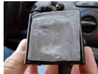
Figure 1.1 Stick double-sided adhesive to base.
