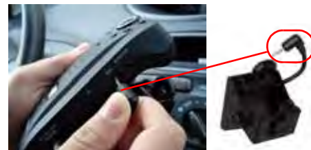
Figure 1.2 Plug minijack into GPS port.
