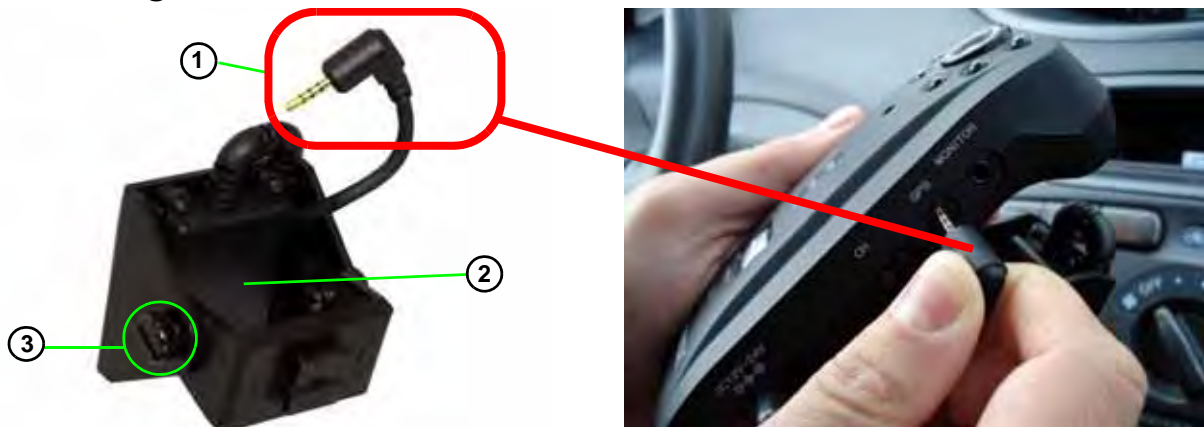
Figure 1.6 Mounting bracket with built-in GPS antenna. Plug GPS mini-jack into the GPS port on the side of the unit.
