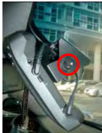
Figure 1.8 Loosen screws to adjust mounting bracket elbow for optimal angle.
