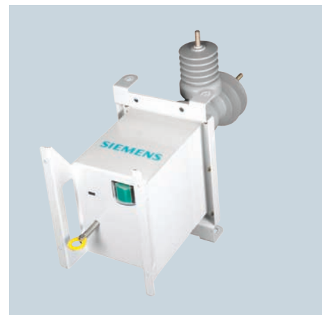
Figure 22: Lockout handle with ring for manual operation (pulled out, recloser open and locked out)
