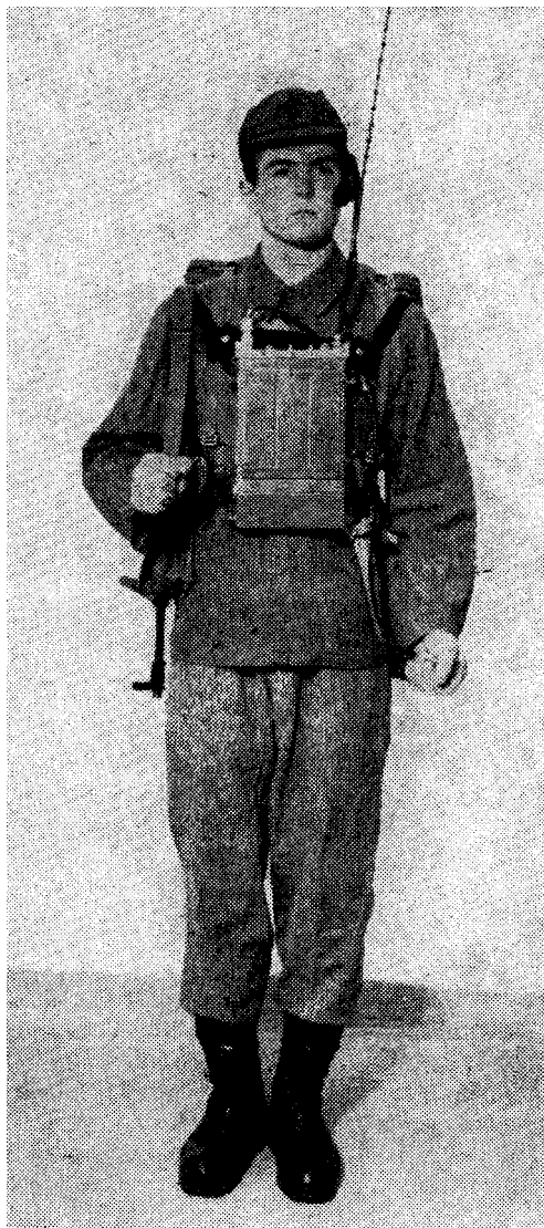
Fig. 77. Soldier with radio station in the "chest" position - with connected rod antenna and headset.
