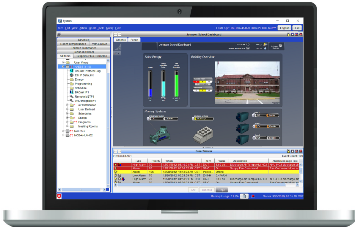
Figure 7: Site Management Portal UI on NAE85
