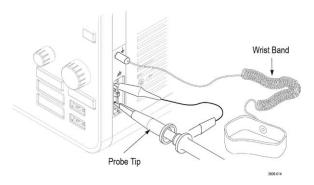
Figure 4: Probe Comp connections.
