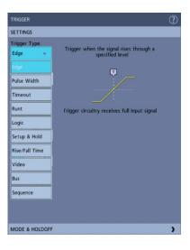
**NOTE.** To trigger on a bus, you must first add the bus to the Waveform view. See Add a math, reference, or bus waveform on page 75
