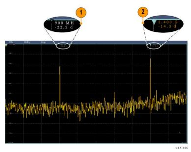
Each automatic marker has a readout associated with it. These can be absolute or delta readouts. An absolute marker readout shows the actual frequency and amplitude of the associated marker. A delta marker readout shows the frequency and amplitude differences from the Reference Marker. The Reference Marker's readout indicates absolute frequency and amplitude, regardless of the readout type.
