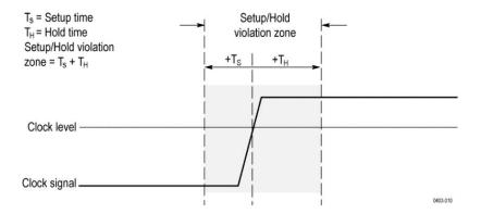
Setup/hold triggering uses the setup/hold violation zone to detect when data is unstable too near the time it is clocked. Each time trigger holdoff ends, the instrument monitors the data and clock sources. When a clock edge occurs, the instrument checks the data stream it is processing (from the data source) for transitions occurring within the setup/hold violation zone. If any occur, the instrument triggers with the trigger point located at the clock edge.
