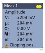
To close the clipping message, change the vertical scale to show the entire waveform, disconnect the probe tip from the excessive voltage source, and check that you are probing the correct signal using the correct probe.
