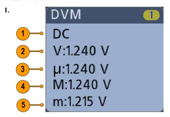
Measurement type (AC+DC RMS, DC, AC RMS, or Frequency)
