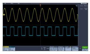
Figure 9: The channel 1 sine wave shows the output of the AFG. The channel 2 square wave show the output of the AFG sync pulse. It comes from the AUX OUT port.
