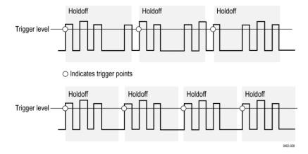
At the longer holdoff time for the top waveform, unstable triggering occurs. With a shorter holdoff set for the bottom waveform, triggers all occur on the first pulse in the burst to remedy the unstable trigger.
