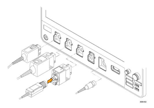
Analog input connectors support all TekVPI+ and TekVPI measurement probes, BNC passive probes, the P6316 Logic Probe, and BNC cables. See *Connecting probes* on page 23.
