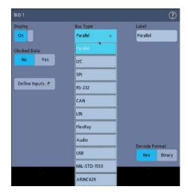
**4.** Use the fields and controls to select the bus signal sources, thresholds, other parameters, and the output format. The following example shows the settings for an I<sup>2</sup>C serial bus.
