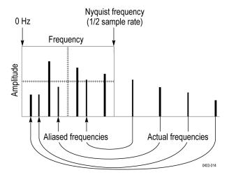
If you have a variable-frequency signal source, another way to observe aliasing is to adjust the frequency slowly while watching the spectral display. If some of the harmonics are aliased, you will see the harmonics decreasing in frequency when they should be increasing or vice versa.
