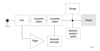
The display shows analog, digital, math, reference and bus waveforms. The waveforms include channel markers and trigger source and level indicators.
