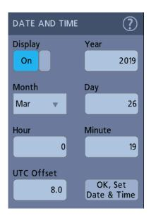
2. To turn off showing the date and time on the screen, tap the **Display** button to **Off**.
