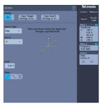
3. Use the configuration menu fields to set the search criteria in the same way that you would set for a trigger condition (select the **Search Type**, **Source**, and conditions on which to search).
