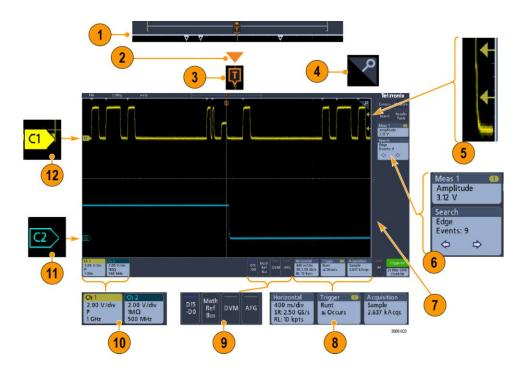
1. The Waveform Record View is a graphical high-level view of the overall acquisition, how much of the acquisition is on the screen (shown in brackets), the location of key time events including the trigger event, and the current position of waveforms cursors.
