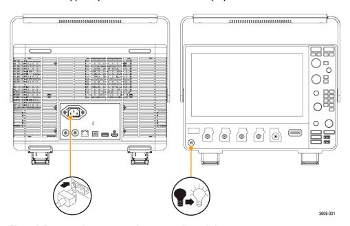
Figure 1: Power cord connector and power standby switch
