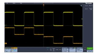
**4.** Double-tap a channel badge to open that channel's configuration menu to check or change settings. See *Configure channel or waveform settings* on page 74.
