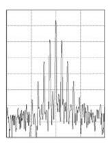
Figure 7: Lower (narrower) RBWs take longer to process, but have finer frequency resolution and a lower noise floor.
