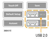
USB ports are located at the lower right corner of the front panel and on the rear panel. Connect USB flash drives to which you can save or recall data (such as instrument software updates, waveforms, settings, and screen captures) or connect peripheral devices such as a mouse or keyboard.
