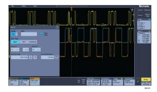
**3.** Use the configuration menus to refine the waveform parameters. Displayed fields depend on the waveform and selections made in the menu. Selection changes take effect immediately.
