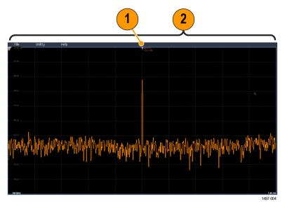
**2.** The span is the range of frequencies you can observe around the center frequency.
