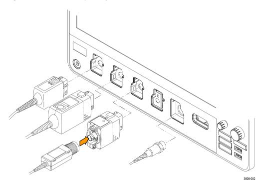
Figure 2: Connecting probes to the instrument
