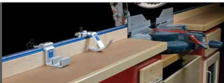
Place 6 feet of Trak on one side and 2 feet on the other side.
