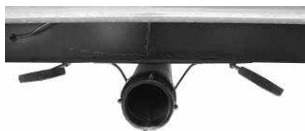
Black/Grey Tank Drain and Valves
