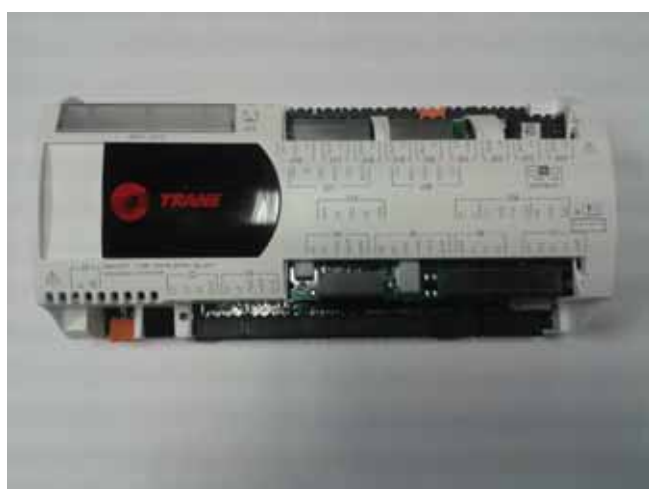
Figure 31 - CH536 main module
