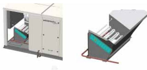
Figure 19 - Heater onto unit and heater detail
